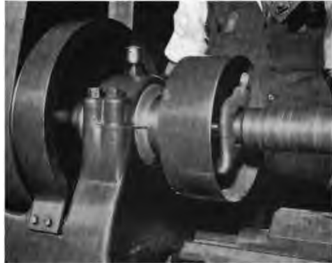
Fig. 2. Guard for Lathe Dog. (Boston Elevated Railway Company.)
